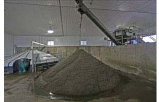
Sand reclaimed through the first phase can be used immediately for bedding. In-floor heating helps dry the sand quickly.
