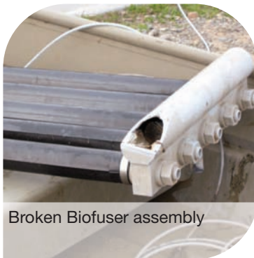
Air leak in the previous style float
