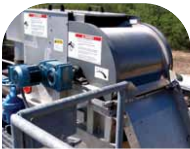
Screens discrete solids, scum and oily materials without blinding
